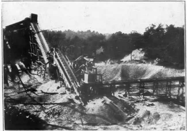
Conveyor at Right Comes from Pit, Center Conveyor to Scalping Screen Conveyor in background to Sizing Screens
